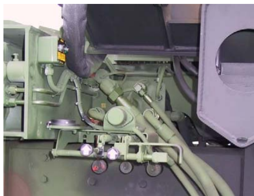
Right hand stabilizer control panel
